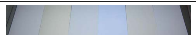
Fig.3. Considered papers in daylight simulator for activation of optical brightening agent effect (fourth from left sample contain the highest amount of optical brightening agent effect) [3].
